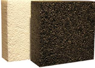
TAC acoustical panels are made with porous, expanded polypropylene bead foam compressed into a dense 2' x 4' panel suitable for ceilings and walls. Class A fire rated, water proof and paintable, TAC combines great acoustical performance and sleek looks with a highly effective tack board surface. TAC can be easily installed with a caulk based construction adhesive and can be cut with basic woodworking tools. TAC is lightweight, mildew and
